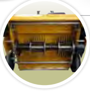
48 all moving knives of hardened steel.
